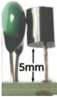
PCB mounting of R11 and Q2
