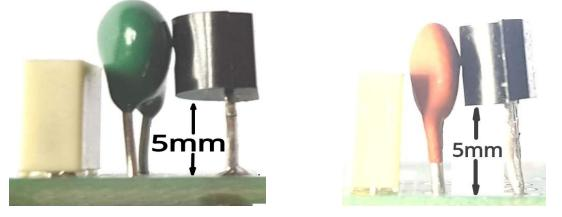
**3.3Assembled PCB:** The finished board should look like the photo on page 1 - check the resistor colour codes and the orientation/polarisation of C1, C2 RV1, Q1-6
