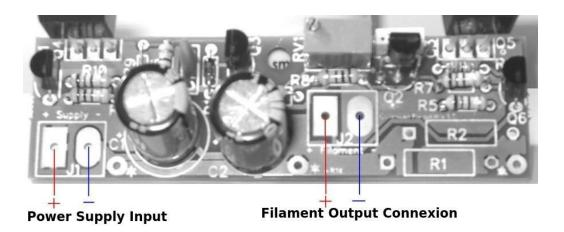
4.16. **Starting the Filament Regulator for the first time.** The Regulator will have been tested with a dummy load (resistor) when you assembled it (See the ASSEMBLY PDF
