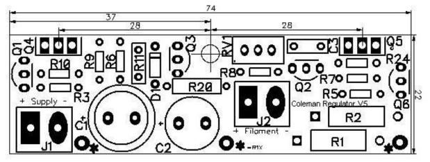
5.2. Drilling and Mounting drawing:
