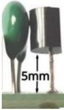
PCB mounting of R11 and Q2
