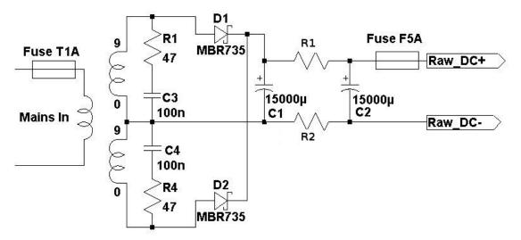
full-wave rectifier, using only two diodes:
