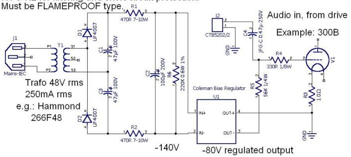
R1 & R2 for filtering and short-circuit protection.
