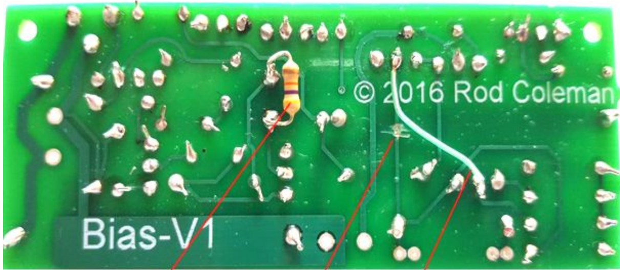
47K across C1 Cut, already made Wire (supplied)
